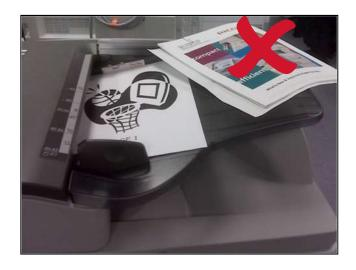
The three sensors on the feed table should not be blocked by paper, etc. It will result in undesired paper size output, or the unit will beep indicating to load special paper size in the tray.
